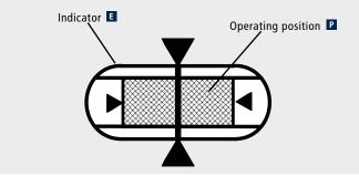
Note: Resetting the pull-rope emergency stop switch must not cause the conveyor system to start up.
